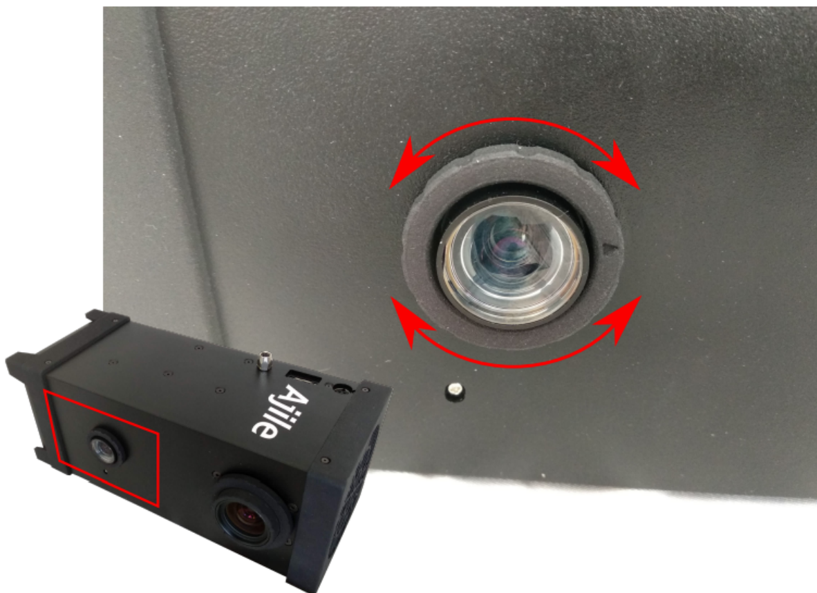
Figure 2.4: Projector focus knob.
