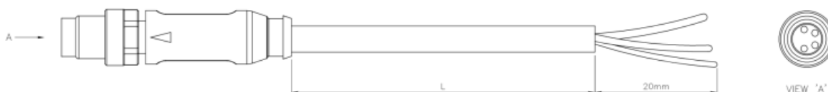
Figure 1.4: M8-4 cable used to connect to DepthScan external trigger interface. TE Connectivity part number 1-2273002-1 shown.
