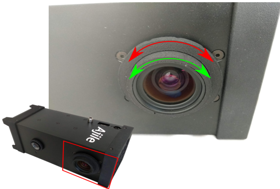
Figure 2.3: Camera focus knob (red) and camera aperture knob (green).
