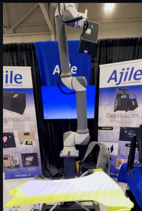
Far position (1 m WD) - robot pulls back for full-part coverage scan of the automotive fender
